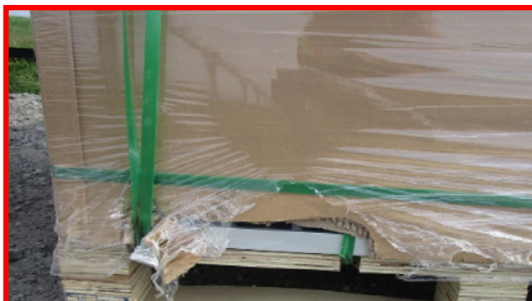
Forklift damage on pallet with exposed modules
